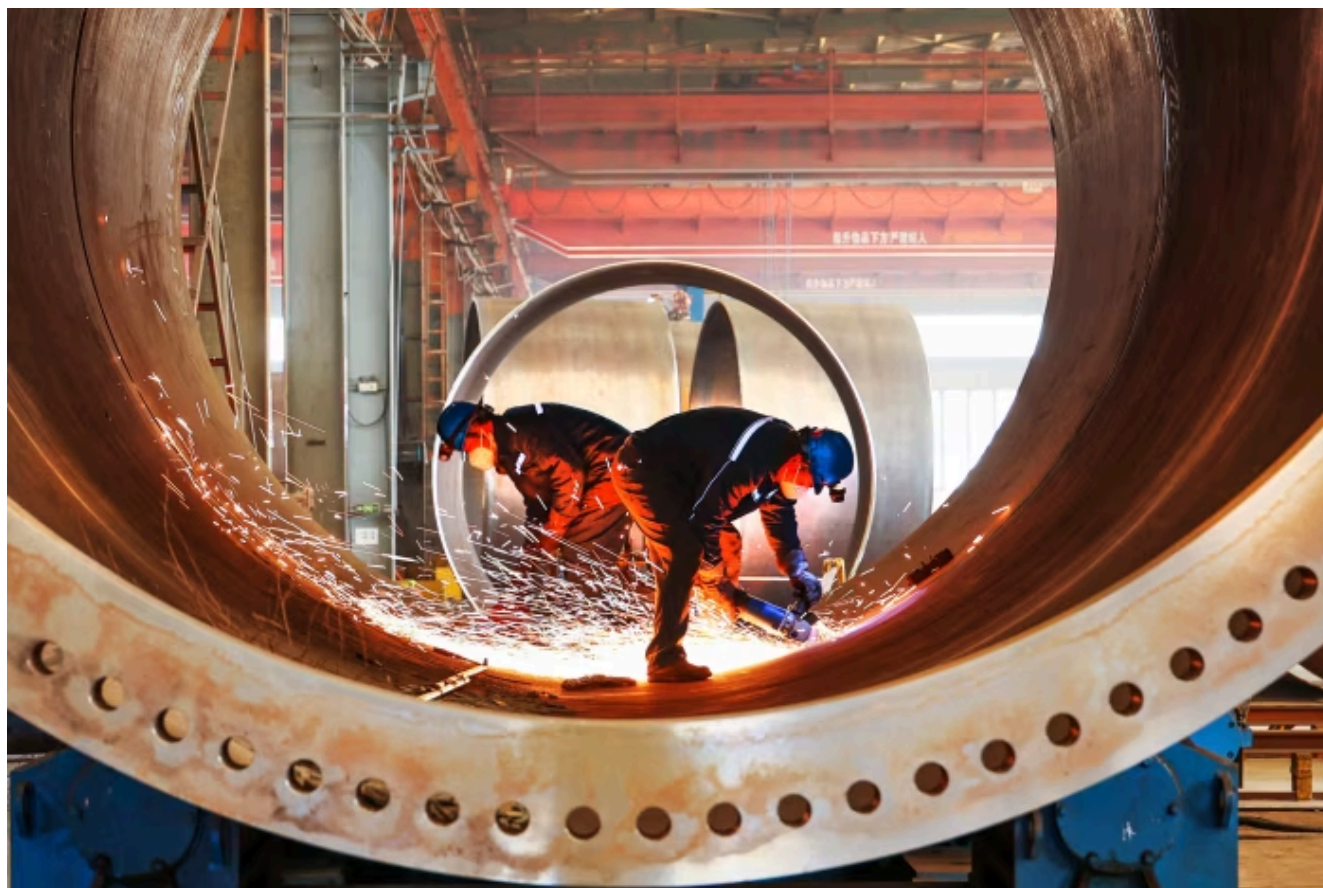
Wind turbine towers being assembled at a factory in China's eastern Jiangsu province © 2025 VCG
